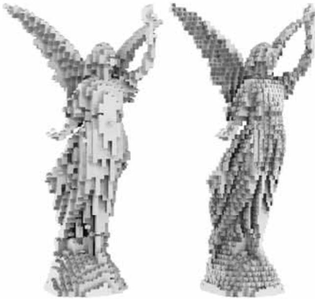
Figure 6: Studs up (left) and studs out (right) versions of a 50cm tall angel statue. Notice the improved detail in the thin sections of folded cloth achieved by reorienting the LEGO pieces.
